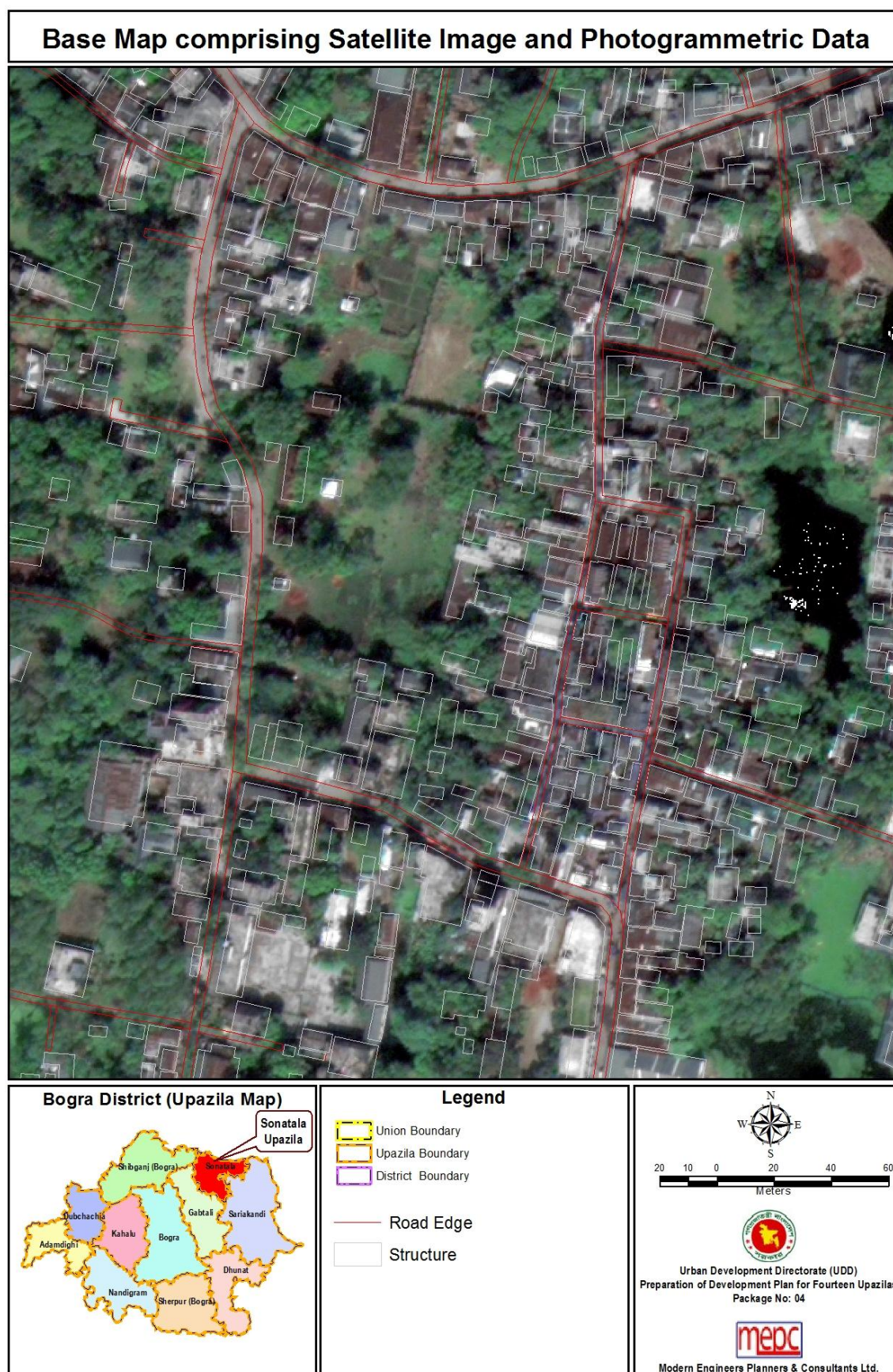
Map 2. 2: Sample Base Map comprising Satellite Image and Photogrammetric Data
