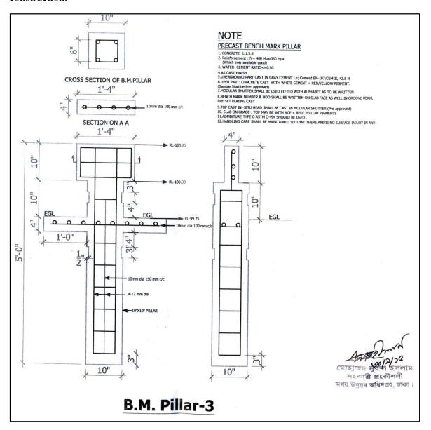
Figure 2. 5: Design of BM Pillars
