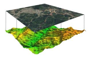
Figure 2. 1: Ortho-rectification of Images
