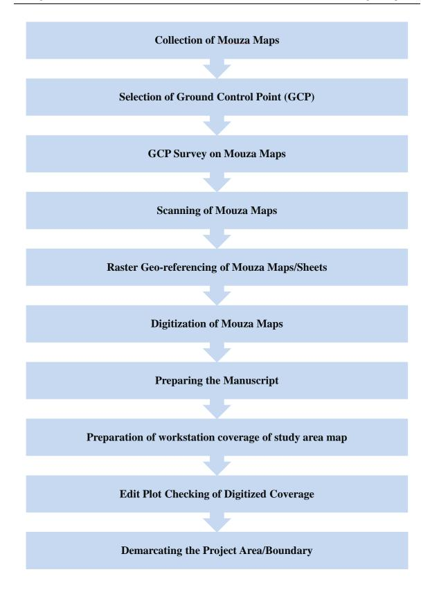
Figure 2. 1: Flow Diagram for Preparation of GIS Database using RS Mauza Map
