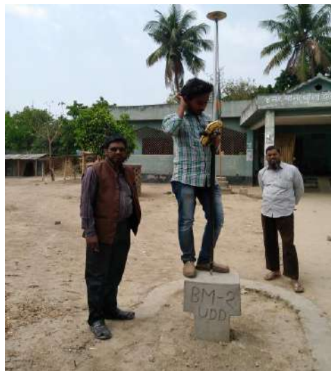
Plate-3: RTK-GPS Observation
