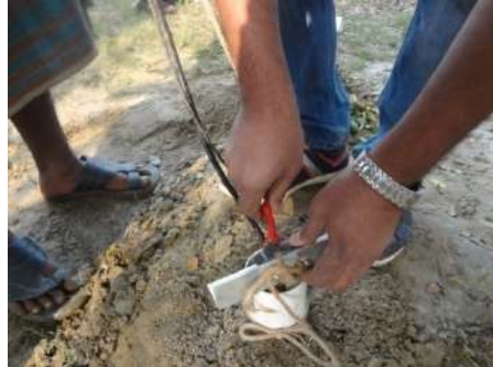
Plate 5: Geophone Lowering In the Borehole
