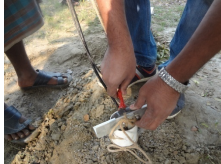
Plate 5: Geophone Lowering In the Borehole
