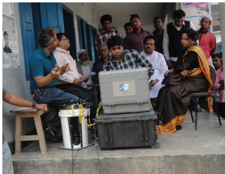
Plate 1: Downhole Seismic Test data logger
