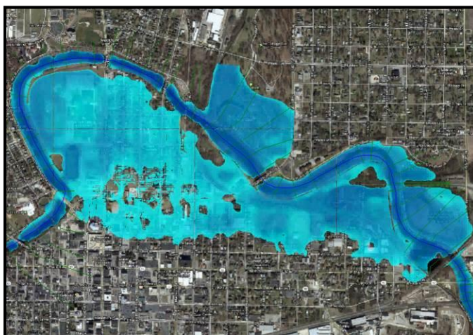
Figure 1.2: An integrated 1D-2D flood model showing flood conditions in a city area using HEC-RAS
