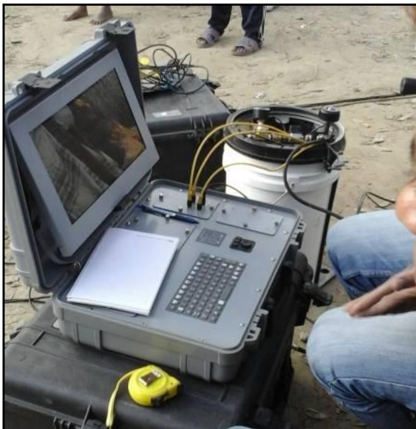
Plate-1: Downhole Seismic Test data logger
