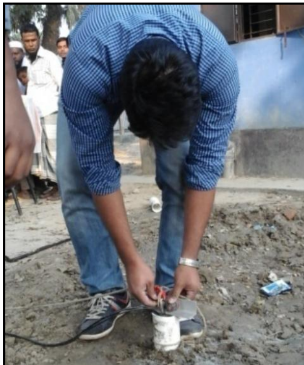
Plate-5: Geophone Lowering In the Borehole
