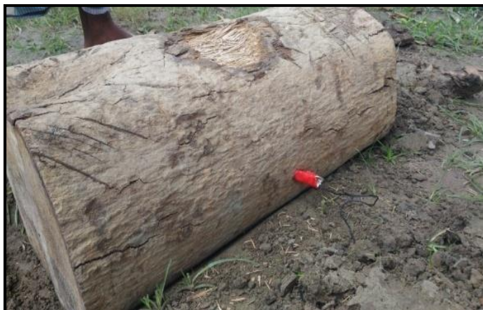
Plate-2: Wooden Plank as the Vibration Source
