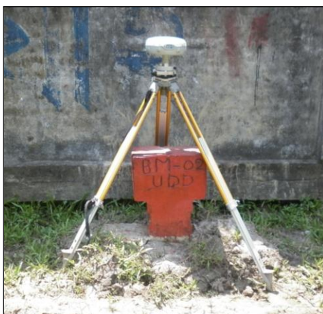
Plate-3: RTK-GPS Observation
