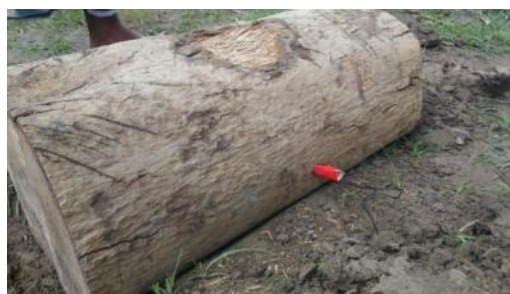
Plate 2: Wooden Plank as the Vibration Source
