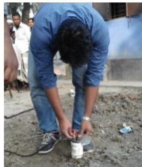
Plate 5: Geophone Lowering In the Borehole
