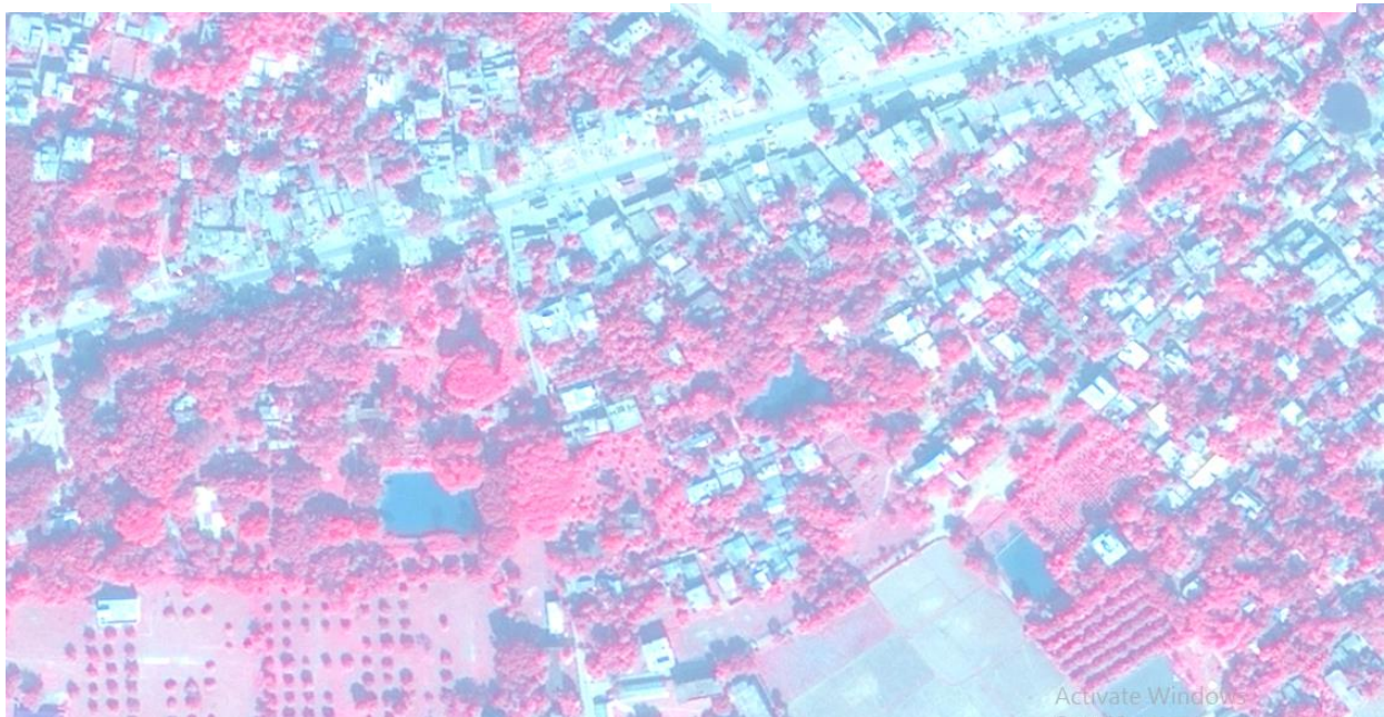
Figure-2.15: Pan-sharpened Image - multispectral 0.5 meter
