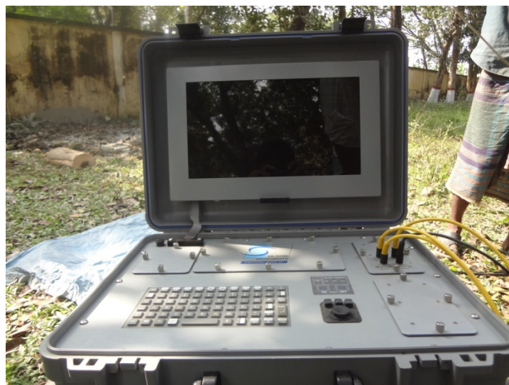
Plate 1: Downhole Seismic Test data logger
