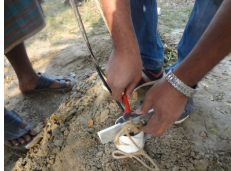
Plate 5: Geophone Lowering In the Borehole
