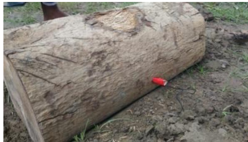
Plate 2: Wooden Plank as the Vibration Source
