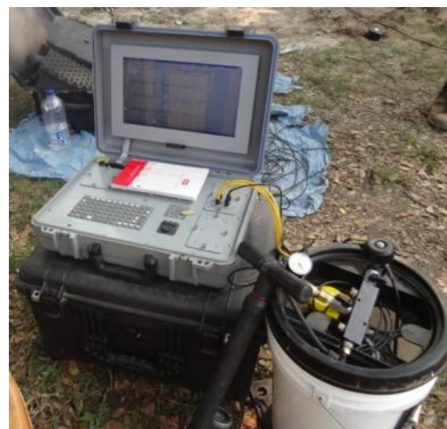
Plate 4: Data Acquisition Unit
