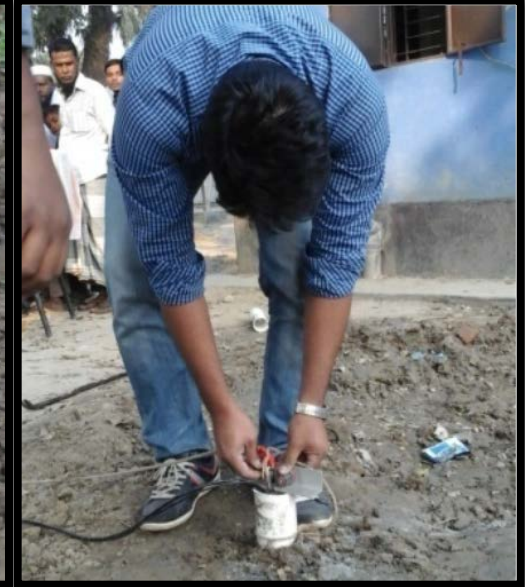
Geophone Lowering In the Borehole
