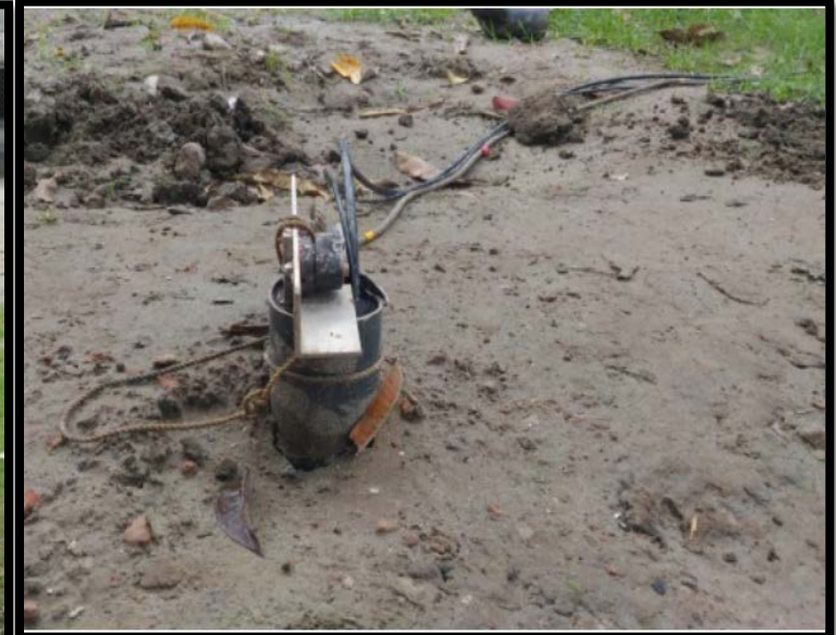
Geophone Installation into the Borehole
