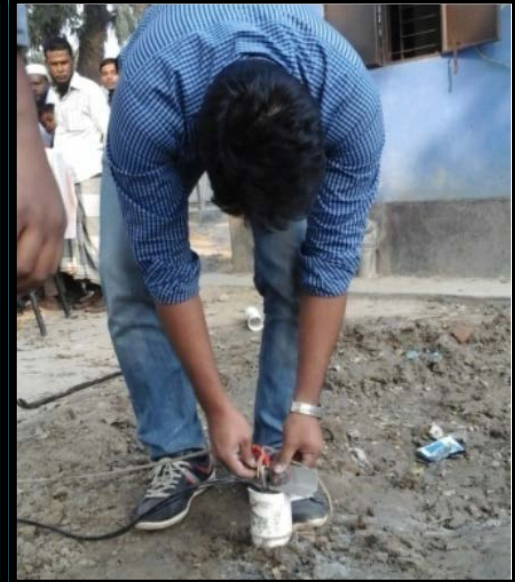
Geophone Lowering In the Borehole
