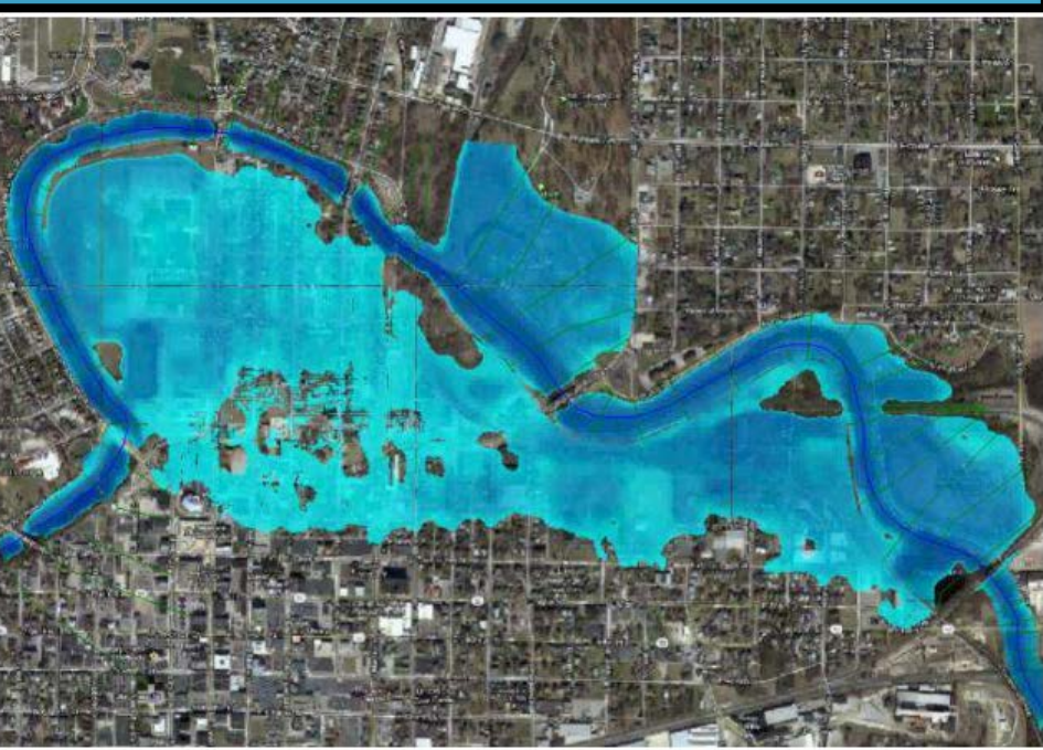
An integrated 1D-2D flood model showing flood conditions in a city area using HEC-RAS
