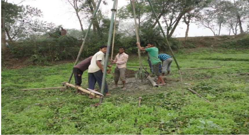
Preparing borehole for Standard Penetration Test
