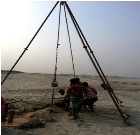
Blowing with hammer for calculating Standard Penetration resistance
