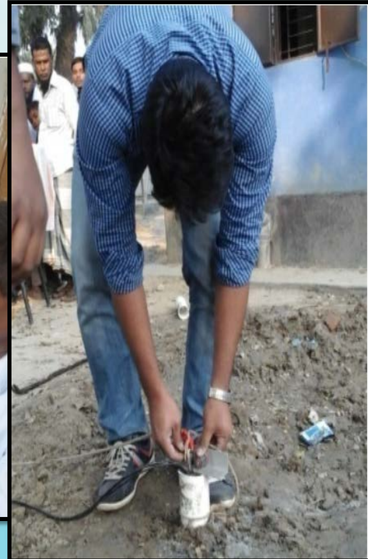
Geophone Lowering In the Borehole
