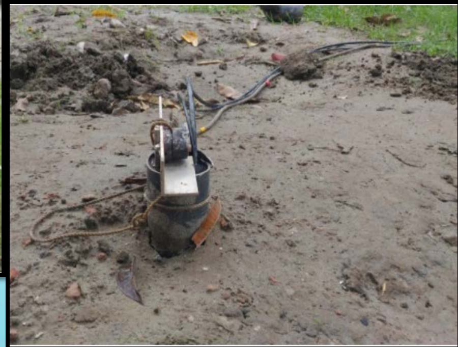
Geophone Installation into the Borehole
