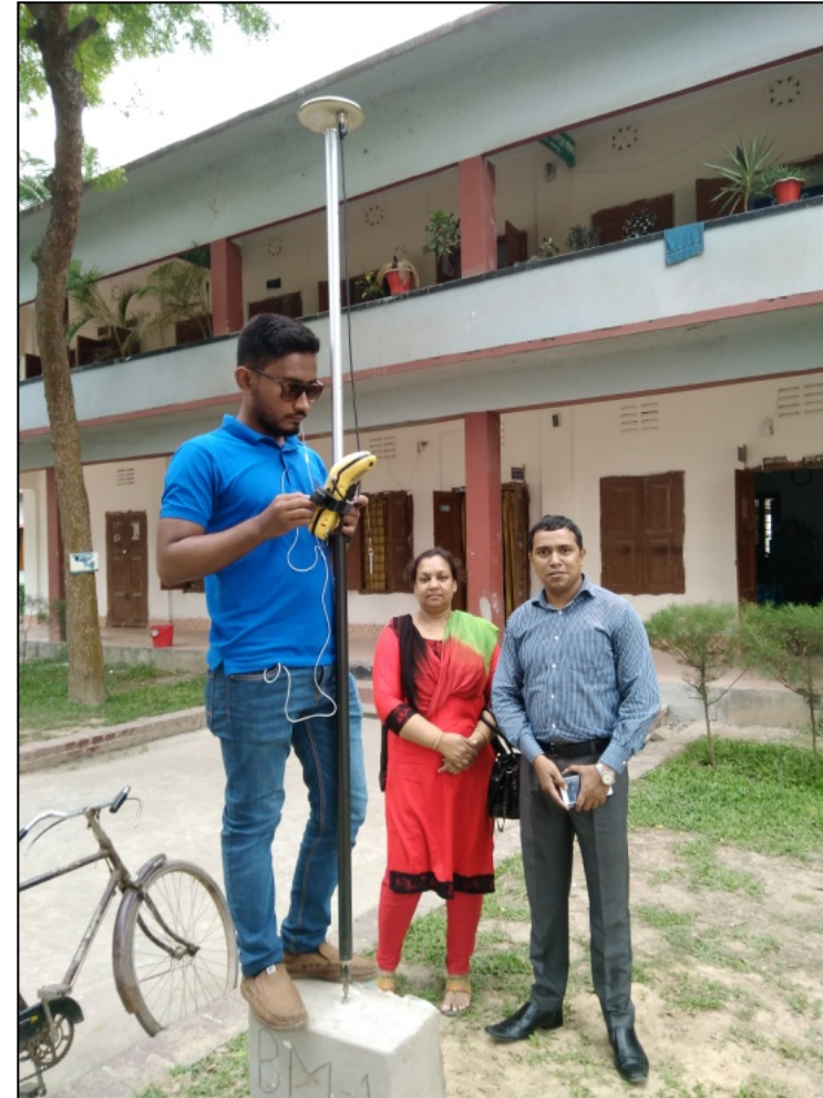
RTK-GPS OBSERVATIONS ON BM PILLARS
