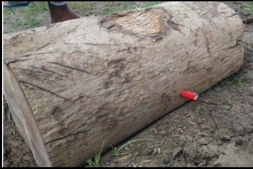
Wooden Plank as the Vibration Source
