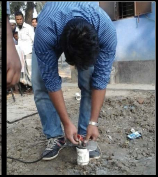
Geophone Lowering In the Borehole
