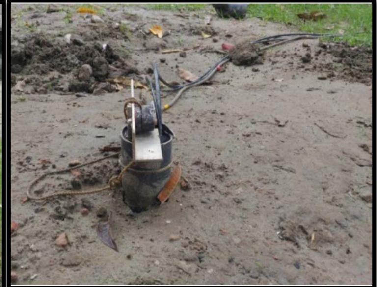
Geophone Installation into the Borehole
