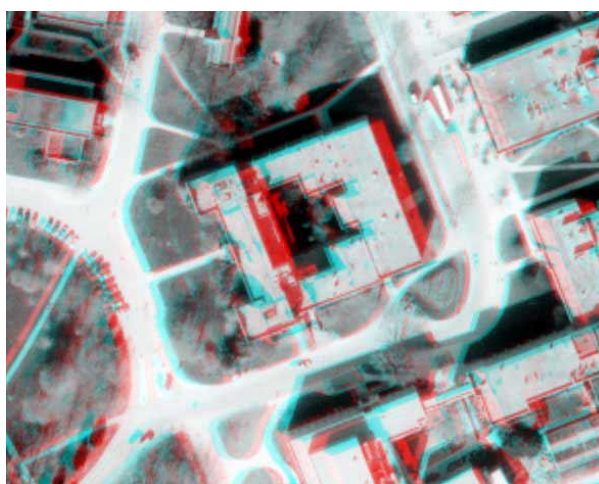
Figure 4.5: Stereo viewing of the overlapping images
